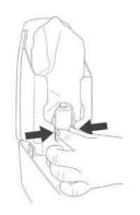
2. Squeeze the nozzle clips to release the pouch
